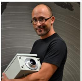
**Above:** Phil shows off one of the new digital cameras ready to be installed in the Desert Fireball Network.
