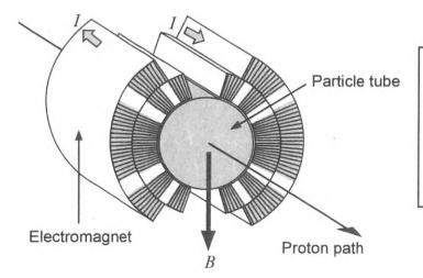
The magnetic field (B) is created by superconductive currents on each side of the tube in which the protons travel. The current (I) moves in opposite directions on each side of the tube.
