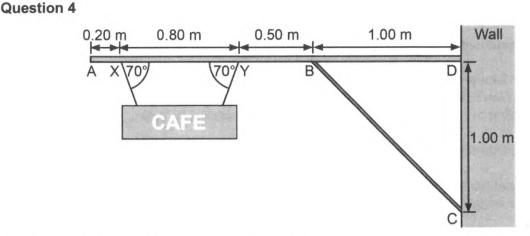
A uniform horizontal 2.50 m beam AD of mass 15.0 kg is attached to the front wall of a shop. It is strengthened and supported by a steel bracket BC that is attached to the beam AD at point B. 1.00 m from end D, and to the wall at point C, 1.00 m below end D.
