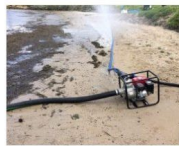
SHORELINE FLUSHING KIT AMOSC EQUIPMENT The shoreline flushing kit is a self-contained, versatile low pressure flushing system for oiled rocky shorelines.
