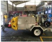
EQUIPMENT WASHDOWN TRAILER AMOSC EQUIPMENT, DECONTAMINATION The Vehicle Washdown Trailer is a semi self-contained trailer designed to prevent secondary contamination from the spill site into the cold zone.
