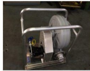
HYDRAULIC AIR BLOWER AMOSC EQUIPMENT, BOOM The HAB 200 is used for in?ating booms. The air blower consists of a hydraulic motor and air blower installed in a portable aluminium frame.
