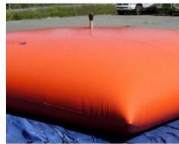
DECK BLADDER AMOSC EQUIPMENT, TEMPORARY STORAGE
