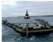
SPEED SWEEP ADVANCED BOOMING SYSTEM, AMOSC EQUIPMENT
